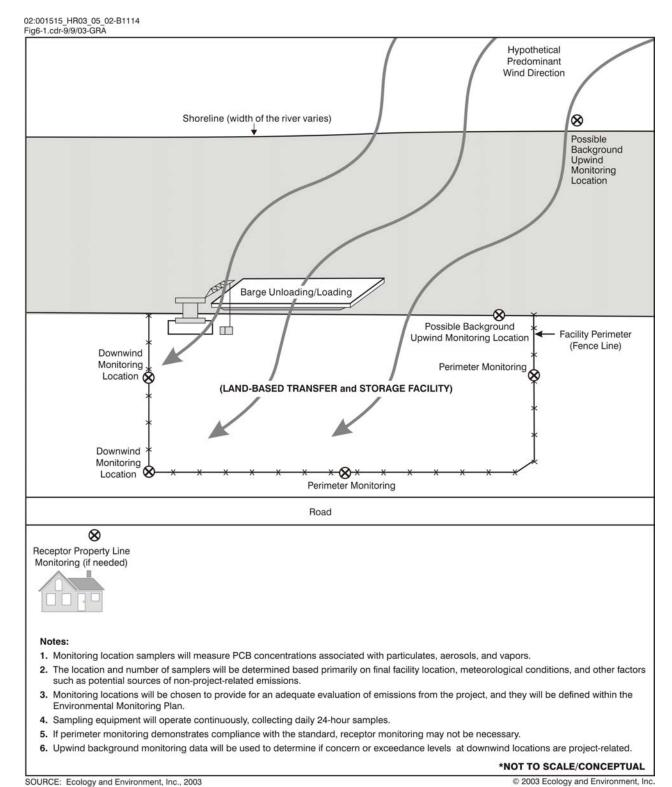
Figure 6-1 Conceptual Air Quality Monitoring Layout: Land-based Transfer and Storage Facility
