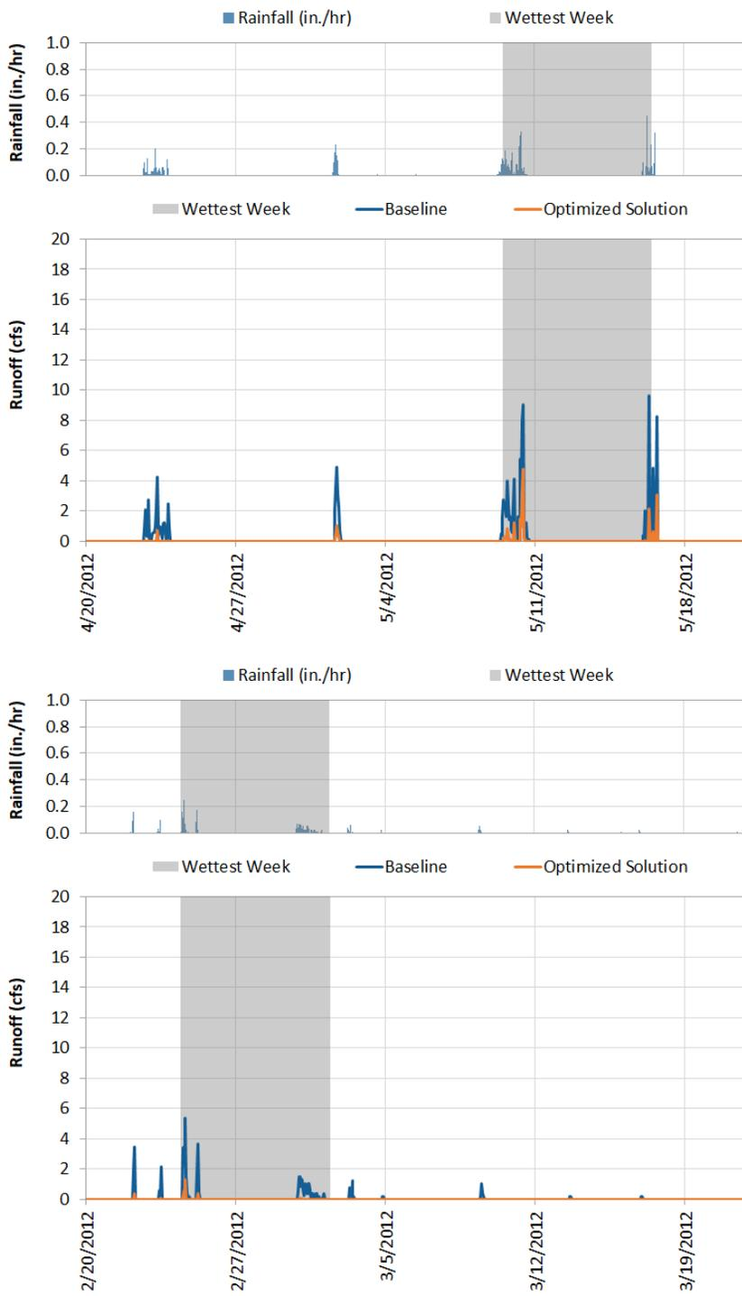
Figure 4-20. Selected periods of rainfall and runoff for outfall #2 during 2012, a year representing an average amount of precipitation for Tisbury, MA.
