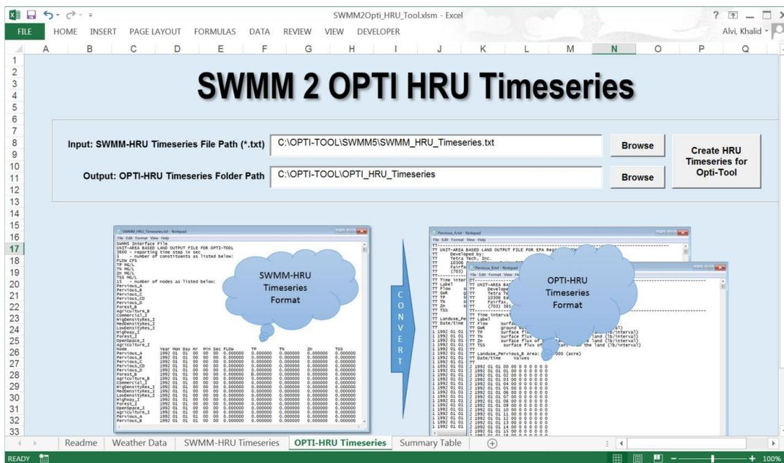
Figure 4-3. The user interfaces for SWMM2Opti-Tool, a utility to reformat SWMM output to Opti-Tool HRU timeseries.
