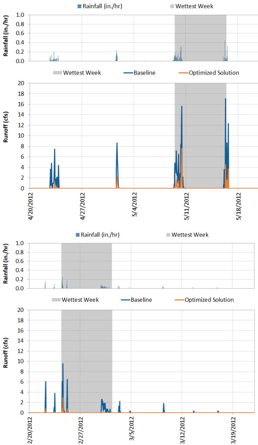
Figure 4-15. Selected periods of rainfall and runoff for outfall #7 during 2012, a year representing an average amount of precipitation for Tisbury, MA. Grey area highlights the wettest week for the period shown.
