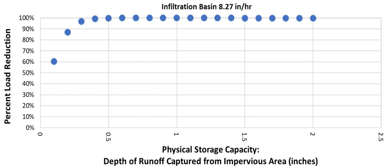
Figure 4-9. Infiltration Basin (8.27 in/hr) performance curve for annual average E. coli load reduction.
