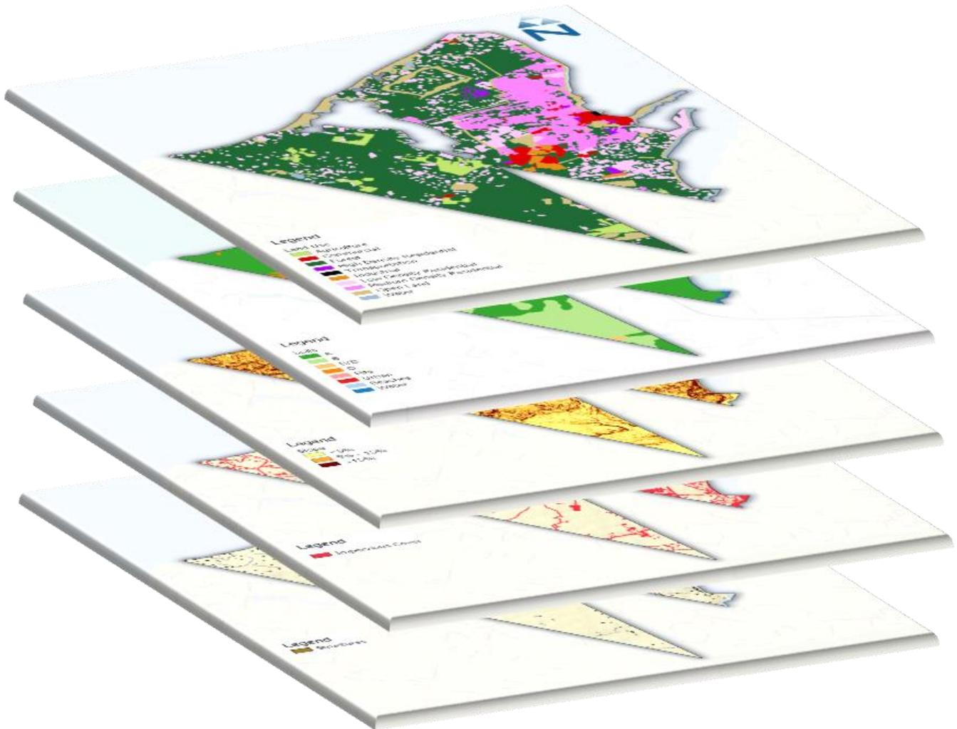
Figure 2-8. Visual representation of the overlaying of land use, soil, slope, imperviousness, and structure layers to create a single HRU layer for Tisbury, MA
