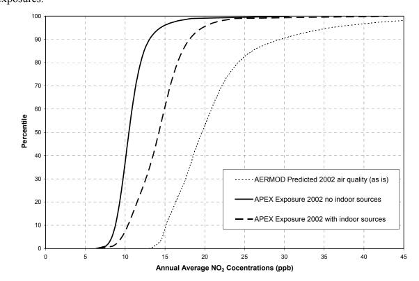
6 Figure B-16. Comparison of AERMOD predicted and ambient monitoring annual average NO<sub>2</sub>
