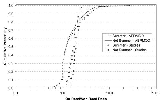
Figure B-14. Comparison of on-road factors developed from AERMOD concentration estimates and those derived from published NO<sub>2</sub> measurement studies.
