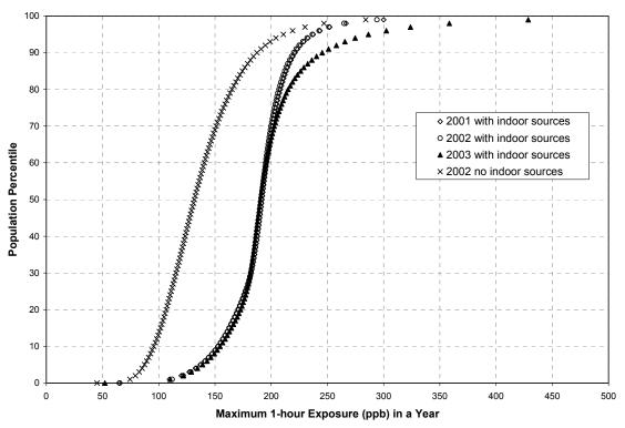
Figure B-17. Estimated maximum NO<sub>2</sub> exposure concentration for all simulated persons in Philadelphia County, using modeled 2001-2003 air quality (as is), with and without modeled indoor sources. Values above the 99th percentile are not shown.
