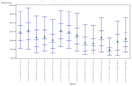
**Figure A-20.** Distribution of hourly NO<sub>2</sub> ambient concentration (ppb) by monitor, Chicago CMSA, 1995-2006.
