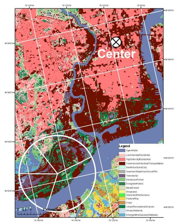
Figure B-2. Land-use and sectors around the Philadelphia-area surface meteorological station (KPHL). Sector borders are 80, 184, 262, and 312 degrees from geographic North. Philadelphia city center is labeled.
