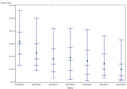
**Table A-72.** Distribution of hourly NO<sub>2</sub> ambient concentration (ppb) by monitor, El Paso MSA, 1995-2006.
