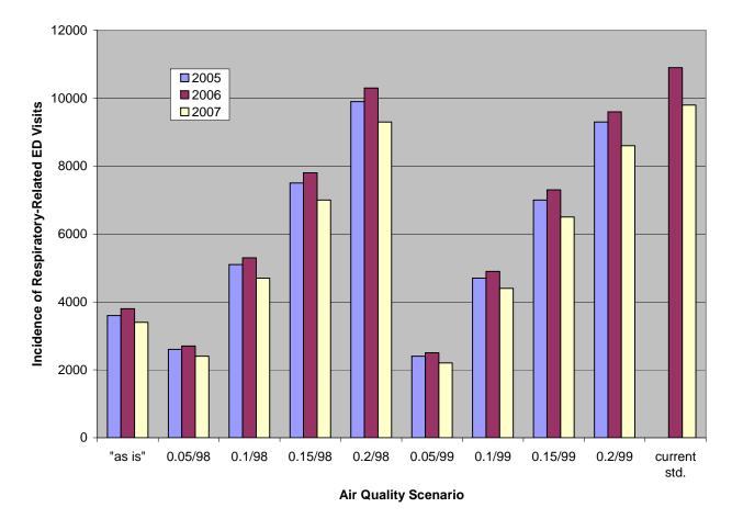
\*The current standard is an annual average standard of 0.053 ppm. Alternative 1-hour maximum daily standards are denoted m/n, where m (in ppm) is the standard level and n is the percentile. So, for example, 0.05/98 denotes a  $98^{th}$  percentile standard of 0.05 ppm. See section 1 for more detail. All results shown are based on the single-pollutant model in Tolbert et al. (2007).
