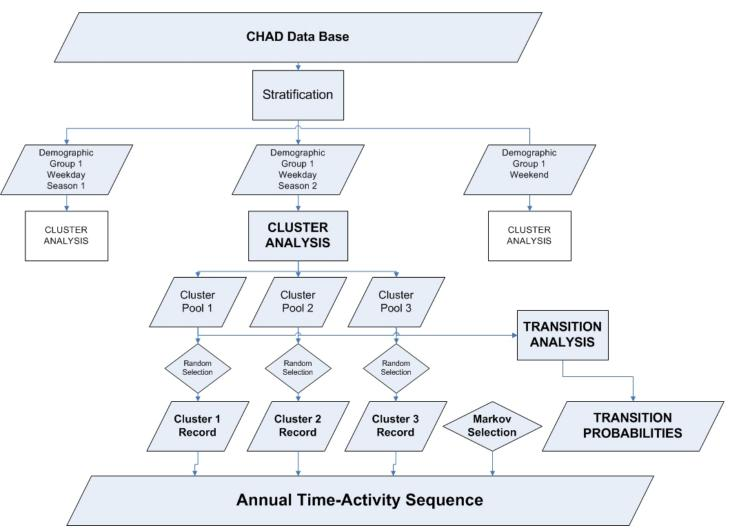
Figure 1. Flow chart of Cluster-Markov algorithm used for constructing longitudinal time-activity diaries.
