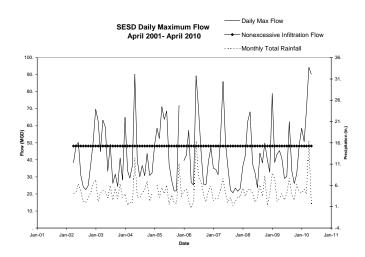
Figures 3 and 4 shows the Average Monthly Flows for the CRPCD and SESD, which exceed the nonexcessive infiltration standard for all but the driest months. This indicates that these systems experience high levels of groundwater infiltration into the system even during dry weather.
