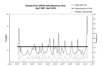
Figure 1. CRPCD Daily Maximum Flow Compared to Nonexcessive I/I Standard
