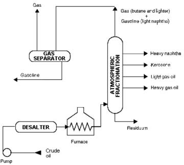
Figure 2-3 Atmospheric Distillation Process
