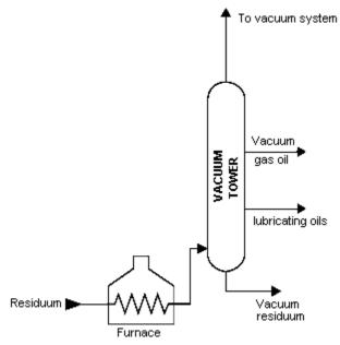
Figure 2-4 Vacuum Distillation Process
