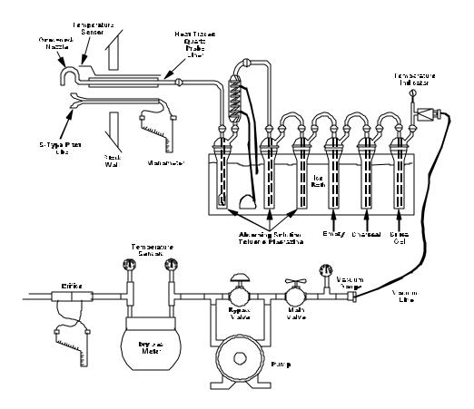
Figure 207-1-1. Sampling Train Configuration for Isocyanates
