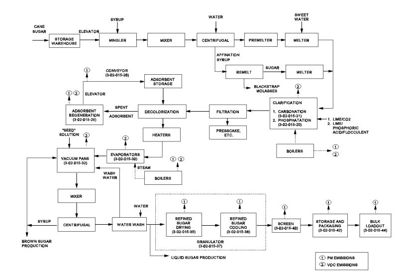
Figure 9.10.1.1-2. Simplified process flow diagram for refined sugar production. (Source Classification Codes in parentheses.)
