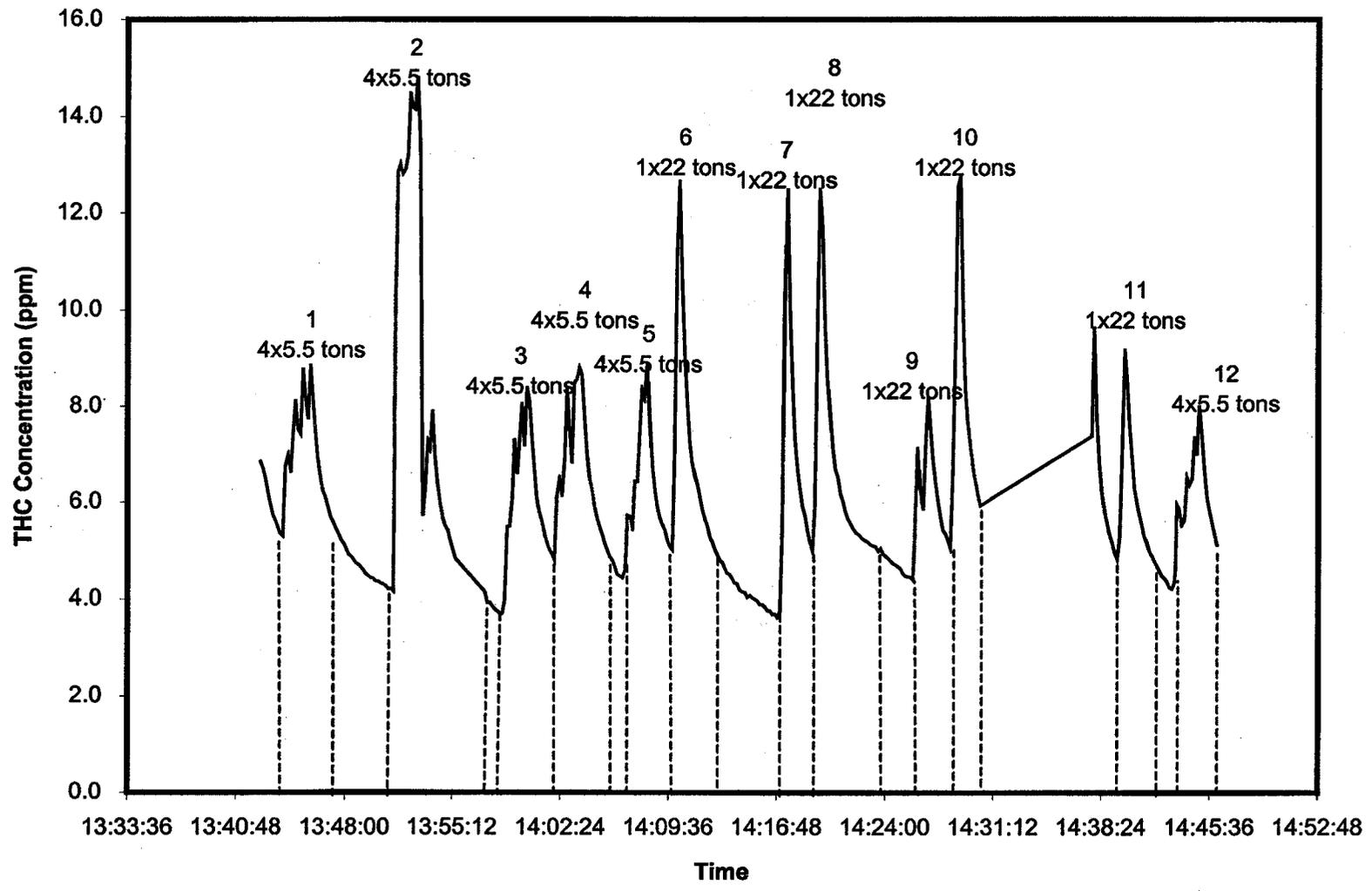
Figure 3-4. THC Concentrations During Intermittent Loadout Testing
