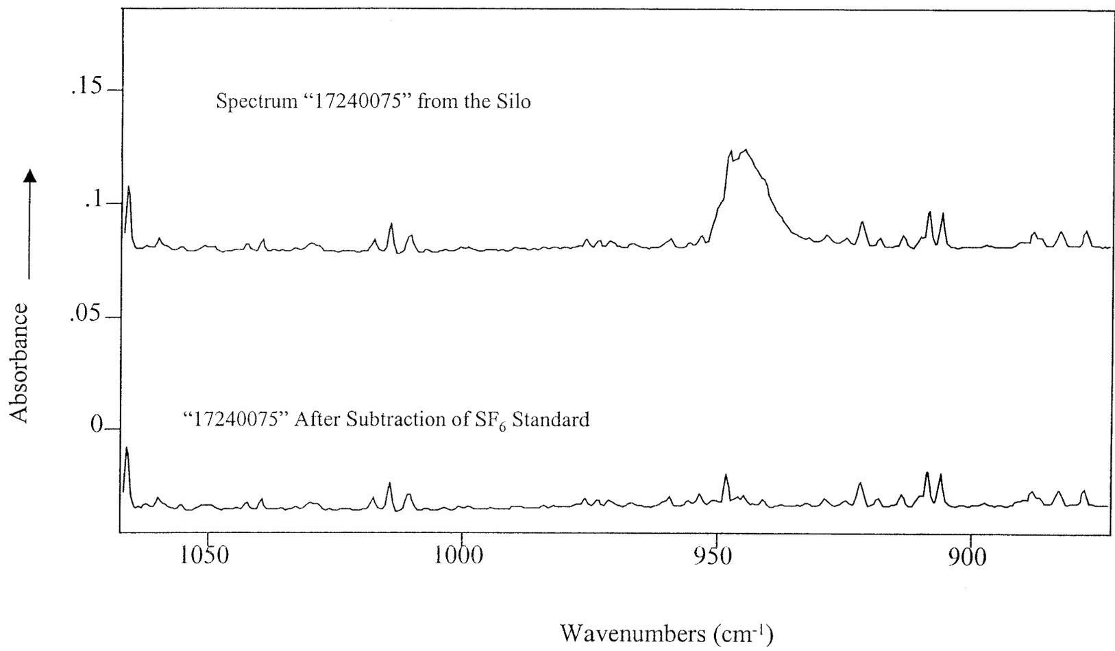
Figure 2. Same Spectra as in Figure 1 plotted on a scale from -.045 to .07 absorbance units. The SF<sub>6</sub> in the top spectrum resulted from the controlled release of the gas standard during testing.
