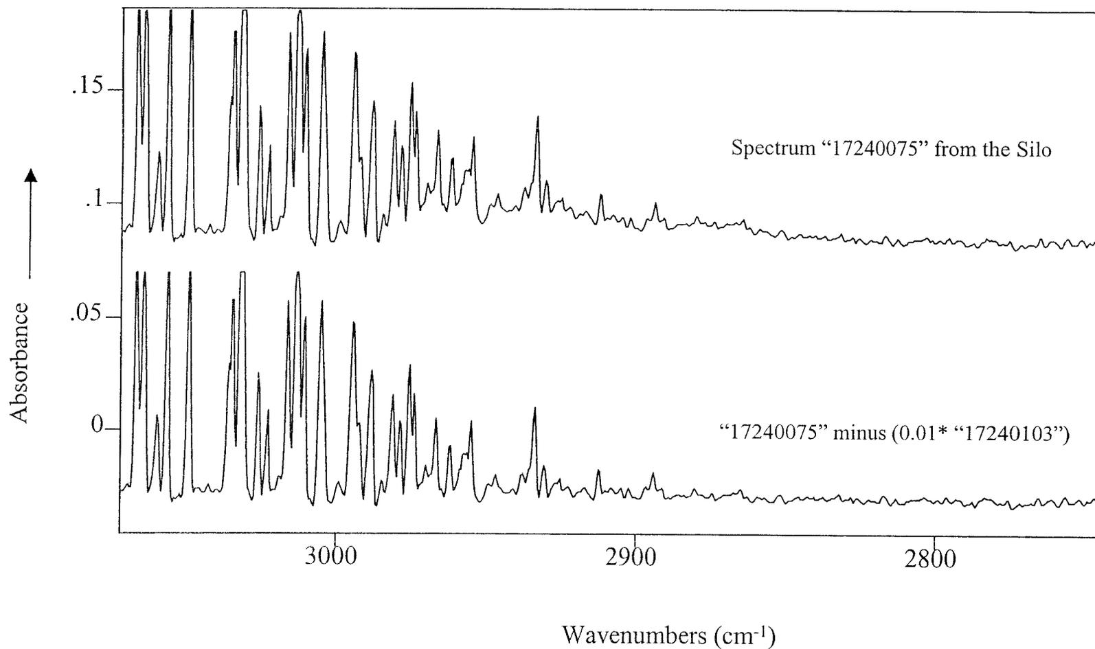
Figure 1. Spectrum before and after hydrocarbon subtraction to prepare for quantitation limit analysis. Both spectra are plotted on the same absorbance scale from -.045 to .07 absorbance units. Note that the water vapor features don't change appreciably after subtraction of the hydrocarbon component.
