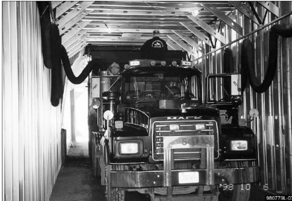
**Figure 7. Truck in Loadout Position - Exhaust Hose Connected**
