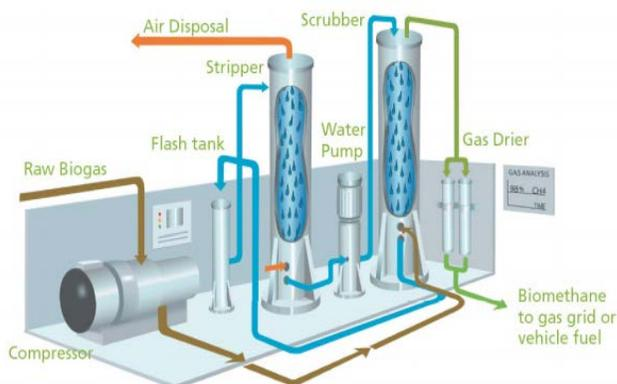
**Figure 7-7. Water scrubbing unit flow schematic.** <sup>22</sup>
