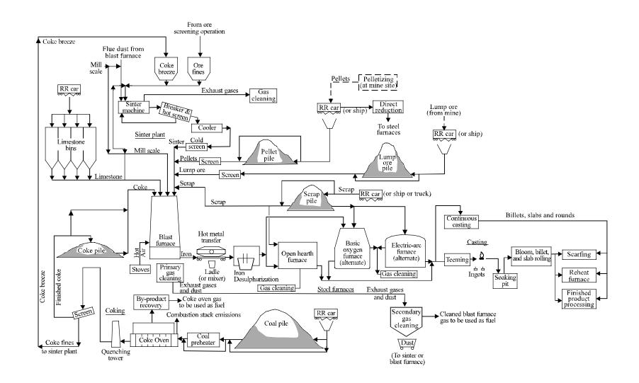
Figure 12.5-1. General flow diagram for the iron and steel industry.
