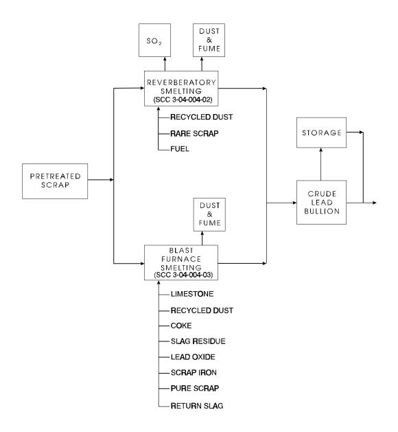
Figure 12.11-1B. Process flow for typical secondary lead smelting. (Source Classification Codes in parentheses.)
