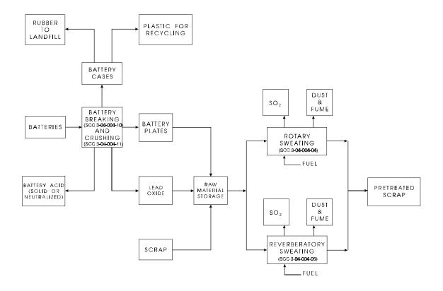
Figure 12.11-1A. Process flow for typical secondary lead smelting. (Source Classification Codes in parentheses.)
