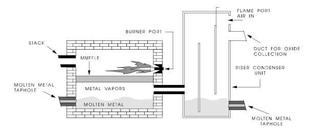
Figure 12.14-3. Muffle furnace and condenser.
