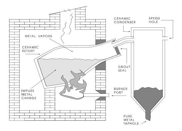
Figure 12.14-2. Zinc retort distillation furnace.
