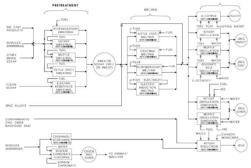
Figure 12.14-1. Process flow diagram of secondary zinc processing. (Source Classification Codes in parentheses.)
