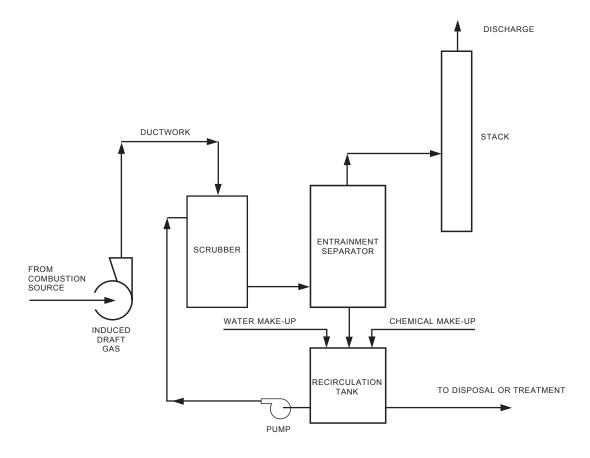
Figure 2.4: Schematic of Venturi Scrubber System
