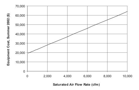
Figure 2.17: Equipment Costs for Jet Venturi
