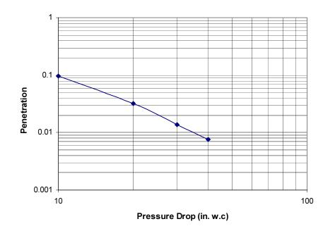
Figure 2.11: Penetration vs. Pressure Drop as Determined from Performance Curves
