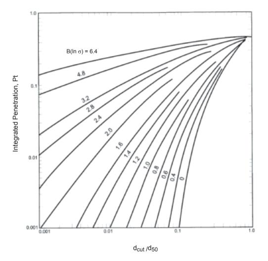
**Figure 2.12**: Cut Diameter as a Function of Cut Ratio and Standard Deviation of the Particle Size Distribution [20]
