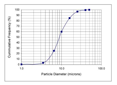
Figure 2.8: Particle Size Distribution for a PM Source
