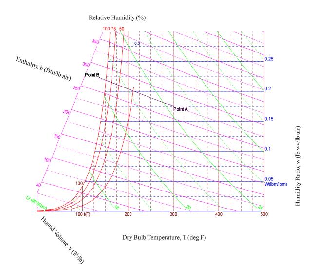
**Figure 2.9:** Psychometric Chart at Standard Pressure, 14.7 psi (Chart developed using Akton Psychrometrics, Akton Associates, Inc.)
