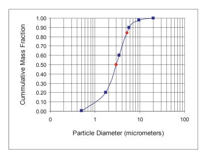
Figure 2.18: Particle Size Distribution for Sludge Incineratior
