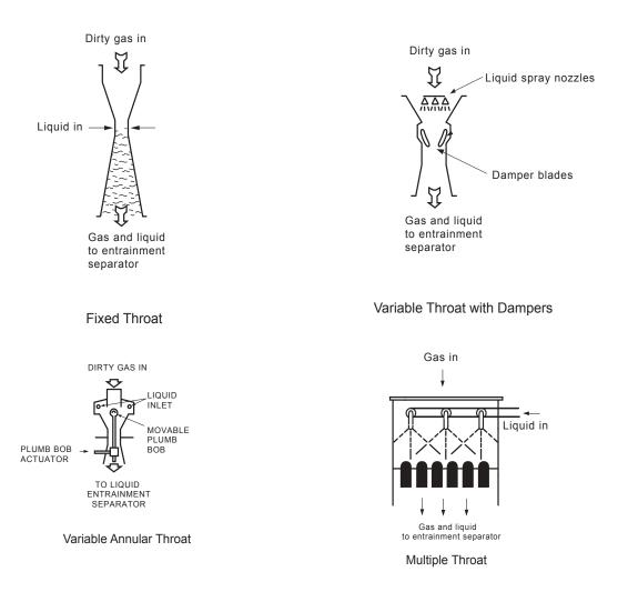
Figure 2.5: Venturi Throat Configurations [9, 11]
