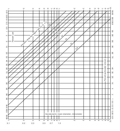
**Figure 2.6:** Approximate Collection Efficiencies of Particles in the 0.1-10 μm Diameter Range at Venturi Pressure Drops in the 6.8-50 in. H<sub>2</sub>O Range [2]
