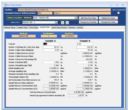
Figure 51 - Paired Sample Train: Sample Data Screen
