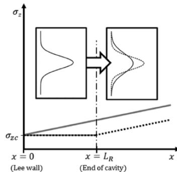
Figure 2. Discontinuity in vertical dispersion ( $\sigma_z$ ) between the re-emitted plume (solid line) and the cavity plume (dotted line) at the cavity boundary ( $L_R$ ). Inset: the vertical concentration profile within the cavity (left panel); the profile after plume is emitted from the cavity (solid line, original; dotted line, revised) (Monbureau et al., 2018).
