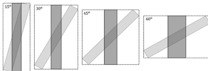
Figure 1. Projected Building using the BPIPPRM Algorithm (Monbureau et al., 2018).
