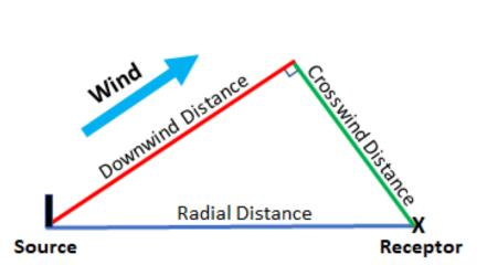
Figure 1. Distance Terms in AERMOD Relative to Source and Receptor Location and Wind Direction
