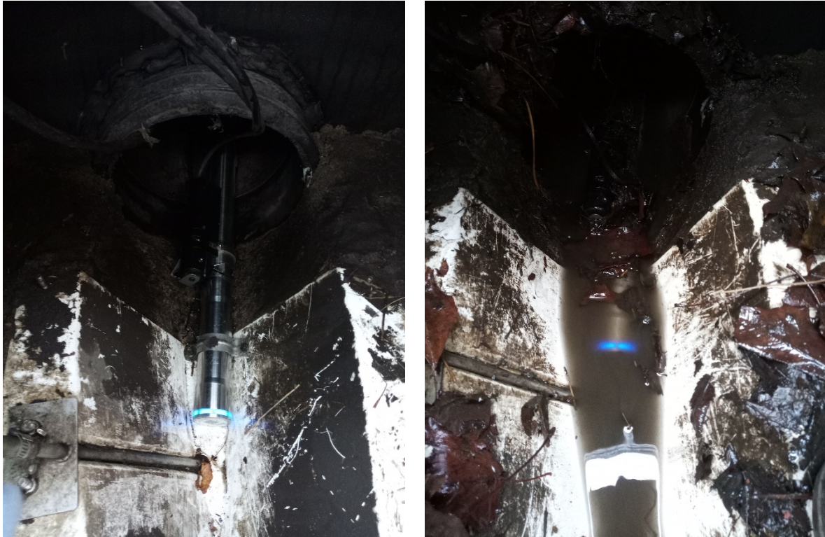
Figure 18: The inlet spectrometer during 2 site visits to illustrate the fouling at the receding limb of the hydrograph.
