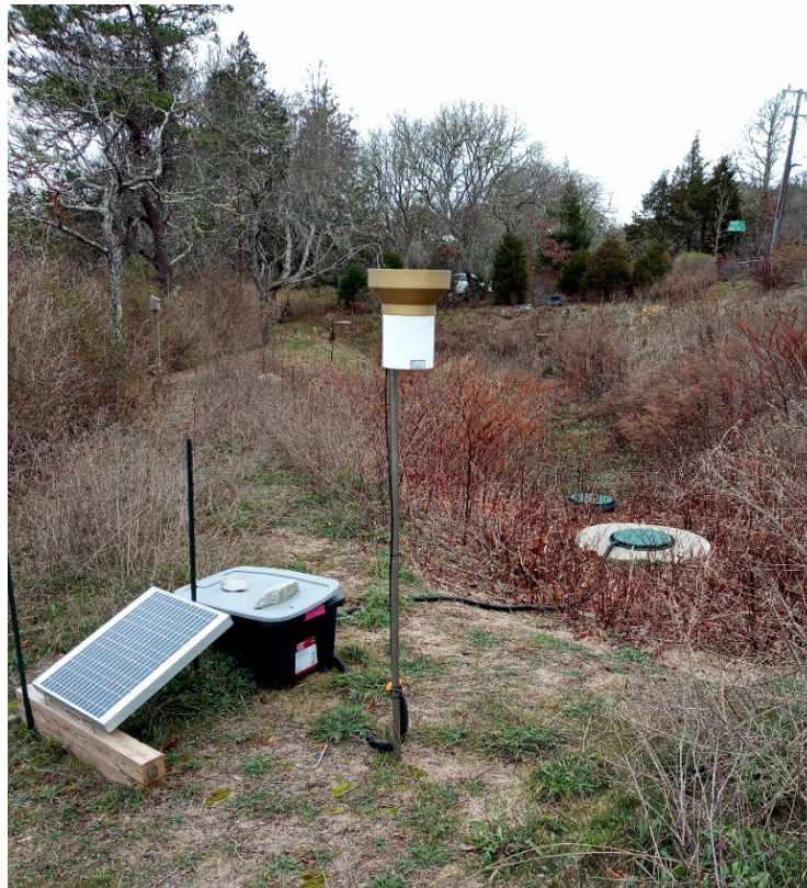
Figure 12: Taken 12/4/20. The effluent monitoring instrumentation included a solar panel, deep cycle marine battery, a tipping bucket rain gage, datalogger, pressure transducer, and UV-Vis spectrometer.
