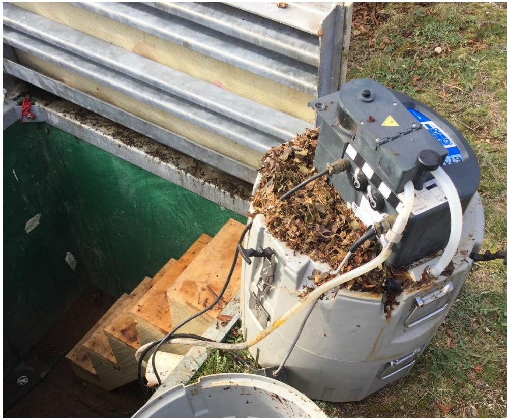
Figure 8: Taken 12/20/19. Outlet equipment infested with mice.
