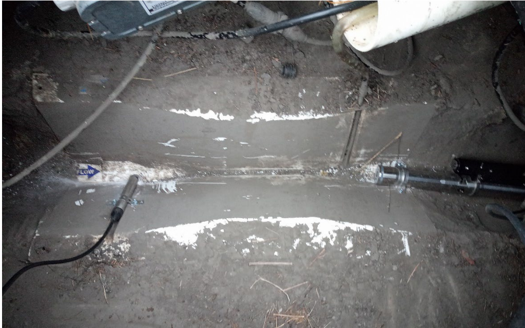
Figure 11: Taken 7/30/20. Inlet instrumentation in the TRACOM Large 60° V Trapezoidal Flume, Campbell Scientific CS 450
