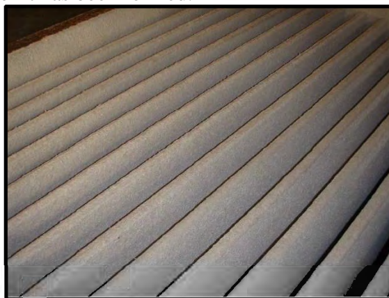
Figure 2-1. Closeup of a Chrysotile Asbestos Diaphragm Outside of the Electrolytic Cell Photograph Courtesy of the American Chemistry Council
