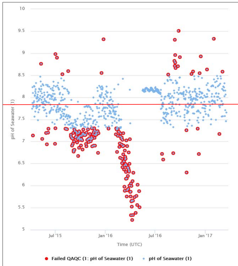
Figure 12 Real time data for pH Coastal Endurance Oregon Offshore Surface Mooring - Near Surface Instrument Frame (44.36485 °N, 124.94343 °W) using the telemetered pH sensor instrument. Note that significant gaps are present in the records. Red circles indicate pH measurements that failed quality accuracy and control. Red horizontal line is pH of 7.8. Current graph can be found at: https://ooinet.oceanobservatories.org/data_access/?search=CE04OSSM-RID26-06-PHSEND000#CE04OSSM-RID26-06-PHSEND000/telemetered_phsen-abcdef-dcl-instrument
