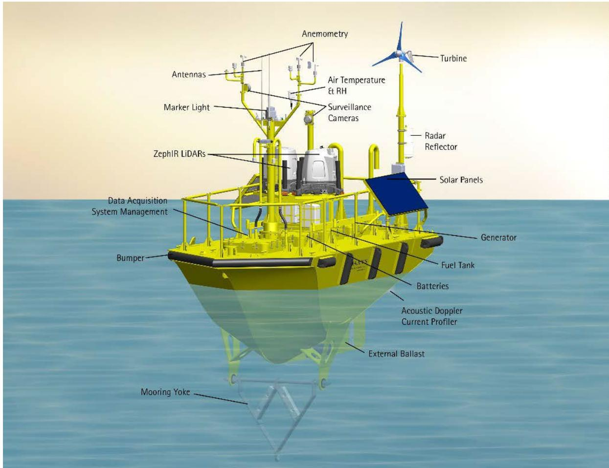
The floating platform consists of the AXYS Navy Oceanographic Meteorological Automated Device (NOMAD) hull, mooring chain, and clump weight anchor. The hull would be moored to the seabed using a steel chain attached to one or two concrete clump weight anchors as shown in Figure 2.
