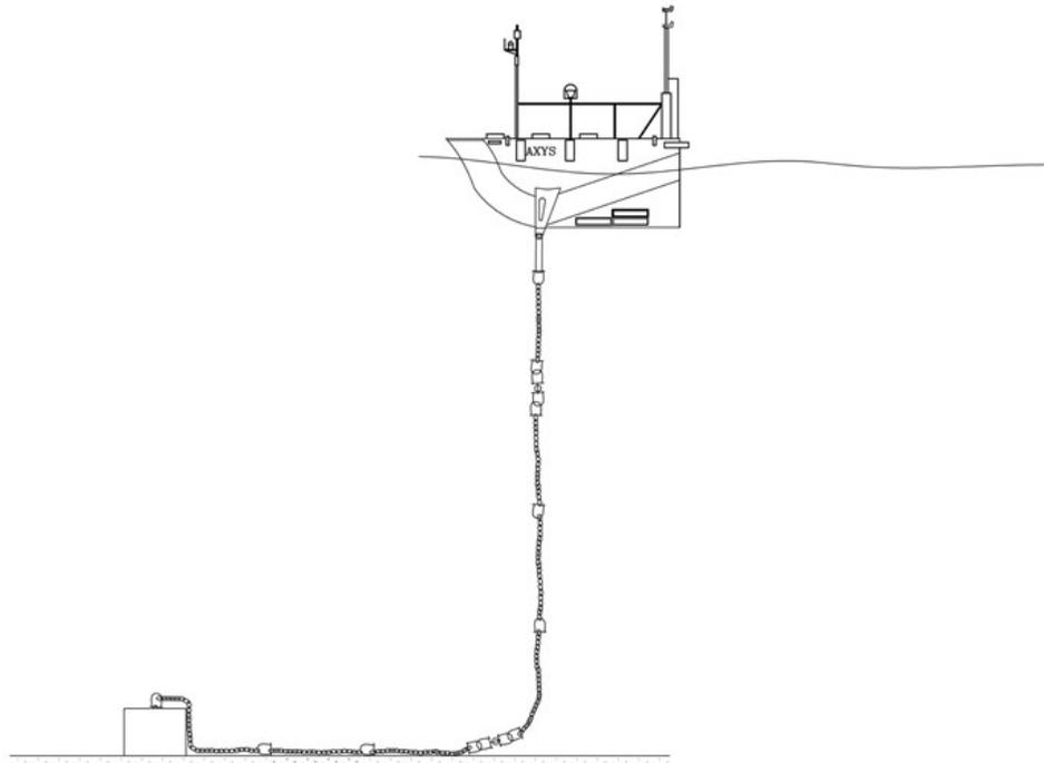
The Met Buoy will be powered by a rechargeable battery pack, which can be charged by an onboard wind turbine, solar panels, or a back-up engine generator. The back-up power will be provided by an onboard 8.5 kilowatt (kW) ultra-low sulfur diesel-fired engine with associated 225-gallon fuel oil tank.<sup>8</sup> The engine will be a Tier 4 EPA-certified engine.<sup>9</sup>
