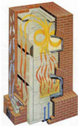
Figure 5. Cross section of a masonry heater. 42
