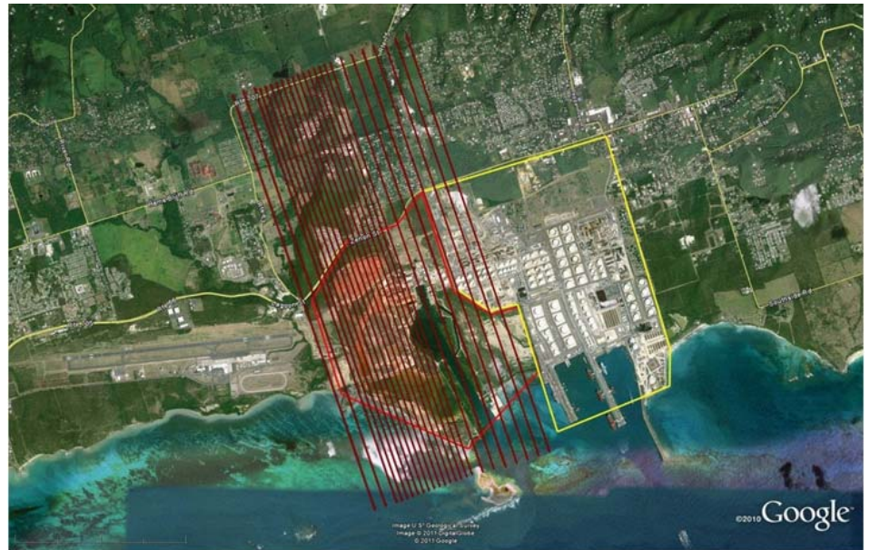
Flight lines for the radiological survey over St. Croix, Alumina site
