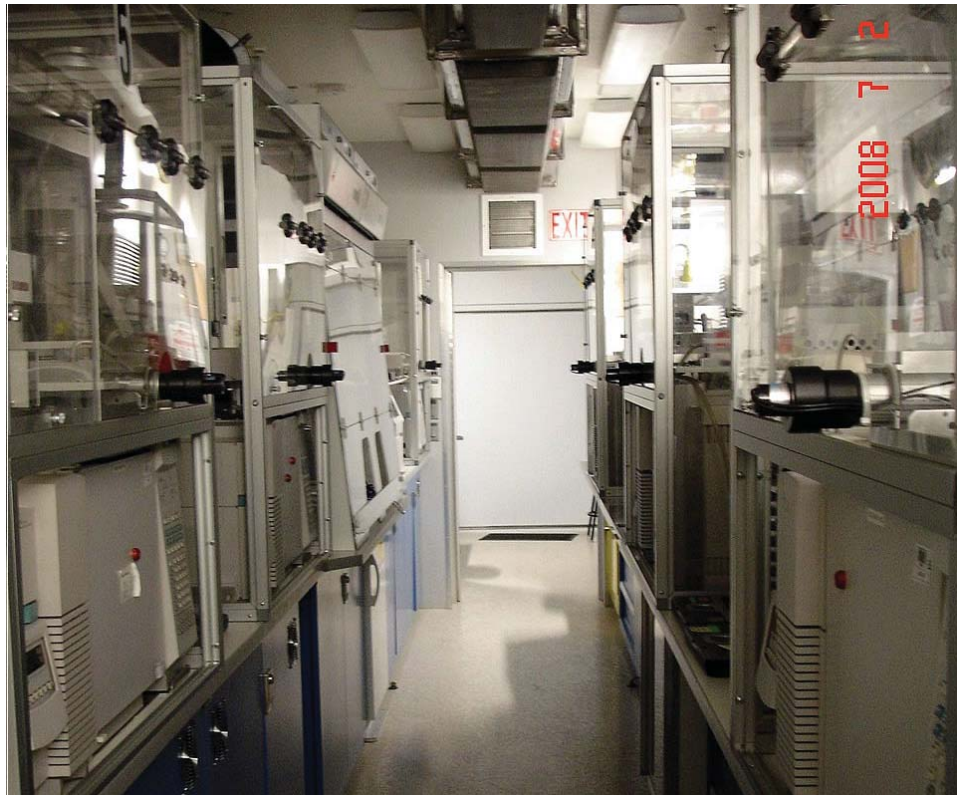
Part of the sample PHILIS log-in station. The metal box is a pass-through for obtaining samples from outside the trailer. The samples are weighed and then bar-coded for tracking in the data system
