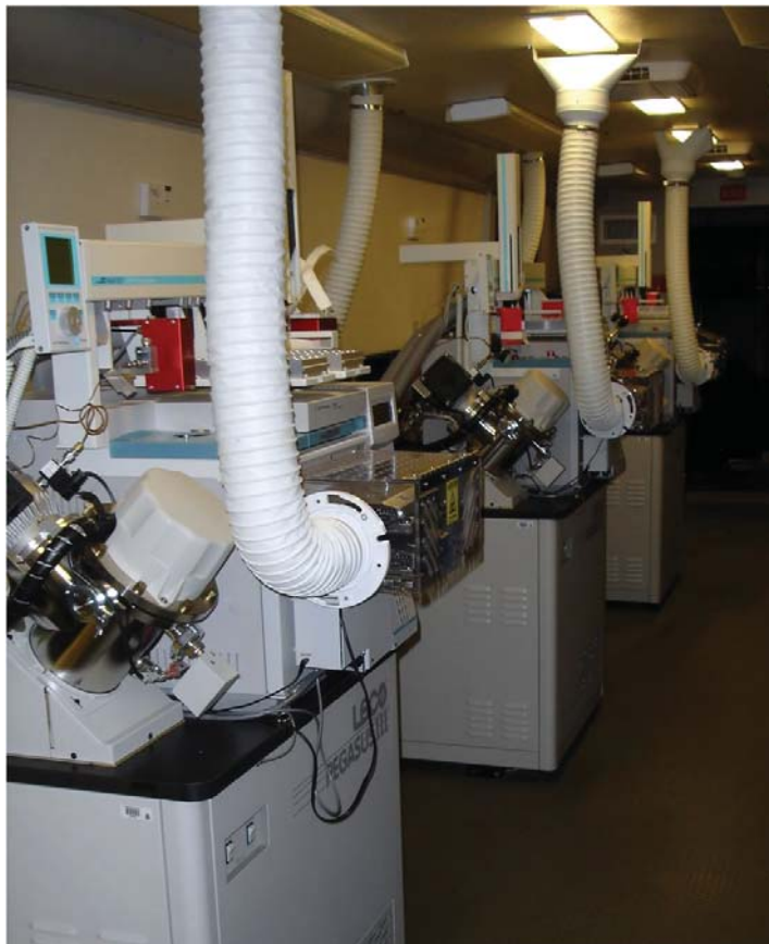
LECO Pegasus III gas chromatograph/mass spectrometer (GC/MS) with an auto-sampling mechanism on top (a Time-of-Flight MS)
