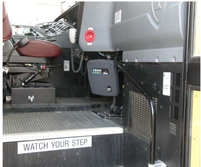
This Adams-12 bus is equipped with a Zonar fleet tracking system device and Z Pass student tracking
