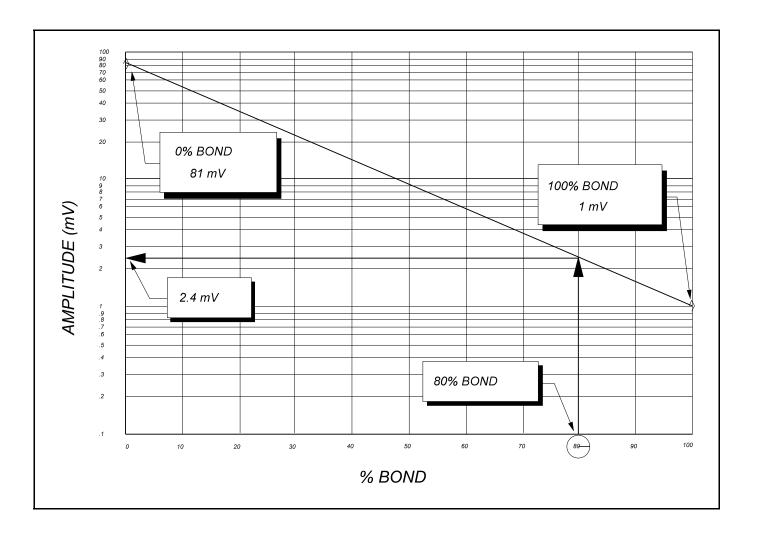
In this example, 80% bond shows an amplitude of 2.4 mV.
