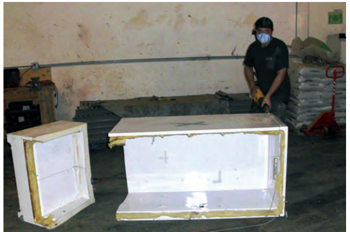
Figure 7: JACO employee removes insulation foam from refrigerator
