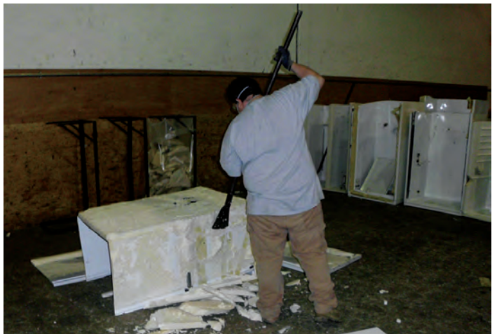
Figure 7: JACO employee removes insulation foam from refrigerator
