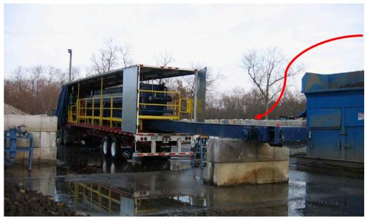
Trailer-mounted Conveyor for cake discharge to container for hauling to disposal
