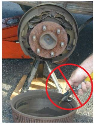
Using compressed air, a brush (wet or dry), or a dry rag to clean brake assemblages has the potential to expose you to asbestos fibers.
