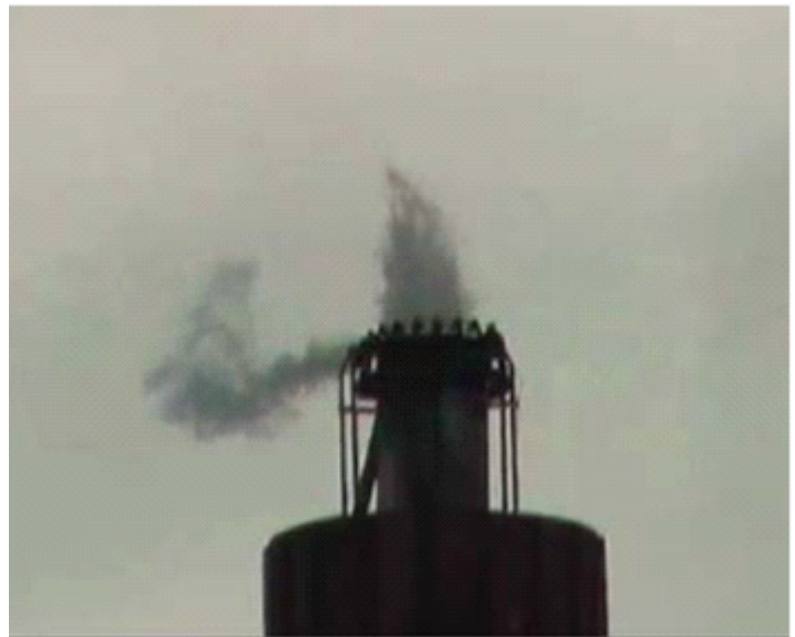
Poorly Operating/Over Steamed Flare - Low Combustion Efficiency
