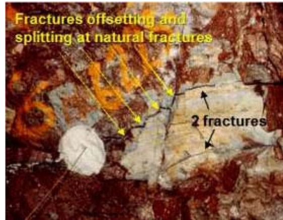
Figure 13. Mineback photograph of offsets & splitting.
