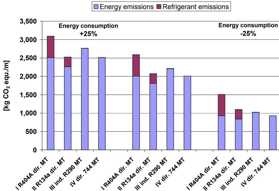
Figure 26: Impact of specific energy consumption upon annual greenhouse gas emissions of the model technologies used by the discounter (leakage rate 6.15%)
