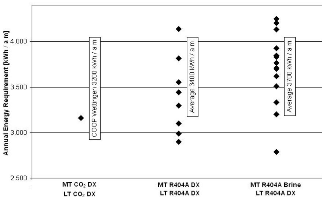
**Figure 11: Energy need per front meter refrigeration unit in Swiss supermarkets. Measured values: COOP Basel, Carrier Kältetechnik Schweiz AG, former LKS Schweiz AG [Heinbokel2006]. Average is based upon best 75 % stores.**
