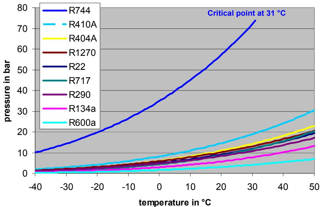
**Figure 6: Vapor pressure curves of refrigerants used in supermarket refrigeration systems calculated with CoolPack version 1.46. In the caption, the refrigerants follow their vapor pressures, i.e. R744 with the highest evaporation pressure at given temperature on top and R600a with the lowest evaporation pressure at the same temperature at the bottom.**
