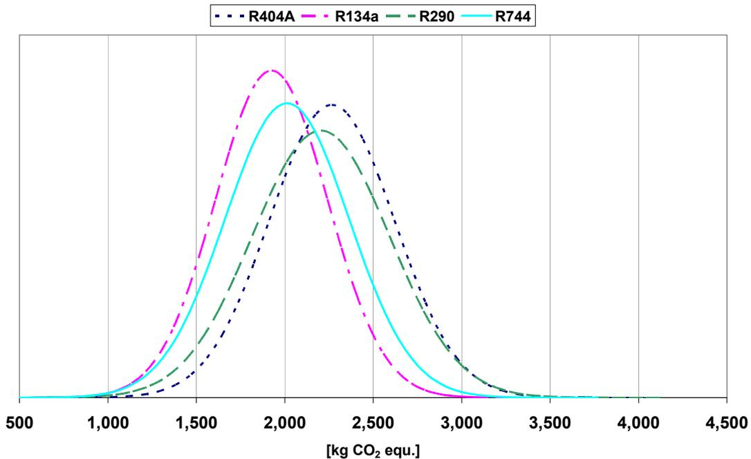
**Figure 8: Probability distribution of annual GHG emissions per linear meter of refrigeration unit for the discounter in connection with different layout options (leakage rate 2.65 % = policy scenario 3) (schematic)**
