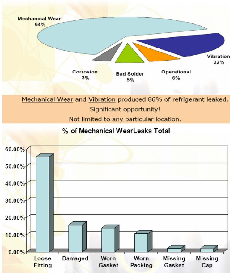
**Figure 19: Refrigerant leakages in central refrigeration systems in the USA [Hoglund2006]. 86 % of the leakages are caused by mechanical wear and vibrations. Under mechanical wear the main part are loose screw joints. Loose fitting consist of flare fittings, Schraeder caps, rotolock valves, service port caps, and others.**
