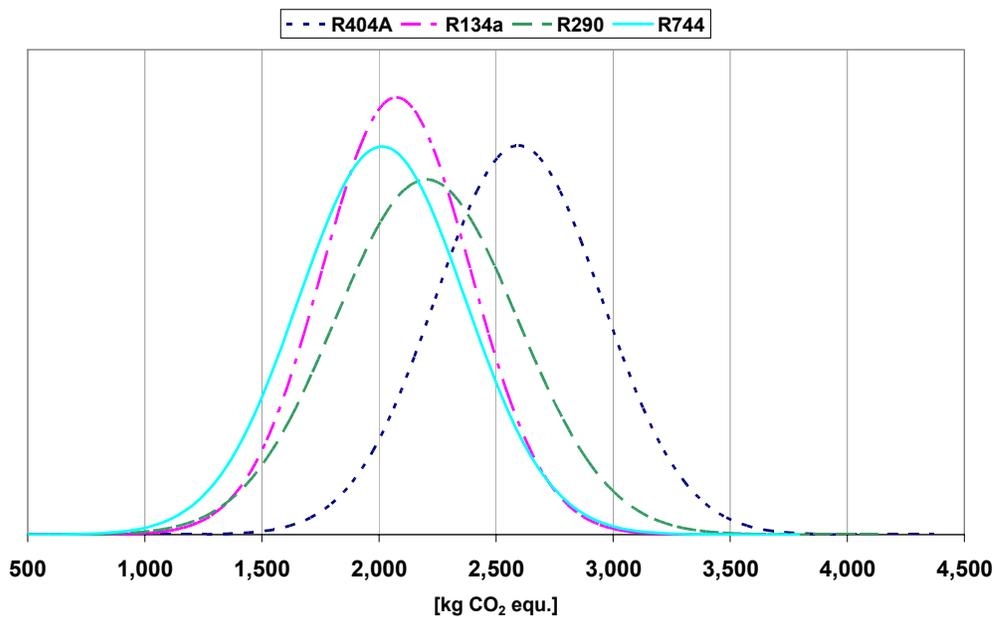
**Figure 7: Probability distribution of annual GHG emissions per linear meter of refrigeration unit for the discounter in connection with different layout options (leakage rate 6.15 % = policy scenario 2) (schematic)**
