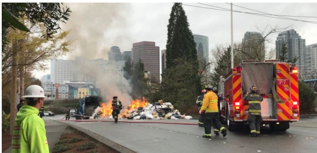
Figure 10: Photo of the aftermath of an LIB fire in a garbage truck. An LIB fire in a garbage truck forced the driver to empty garbage onto the street to be extinguished, disrupting service for customers and creating a traffic hazard for community members and first responders. Photo courtesy of Bellevue Police Department.
