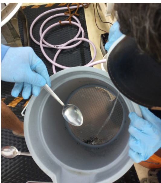
Sediment samples are placed on a sieve and washed to remove sediment and expose macroinvertebrates.
