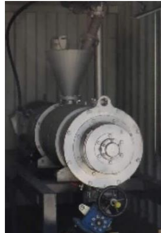
Batch pilot-scale stirred ball-mill, 100 kg batch size
