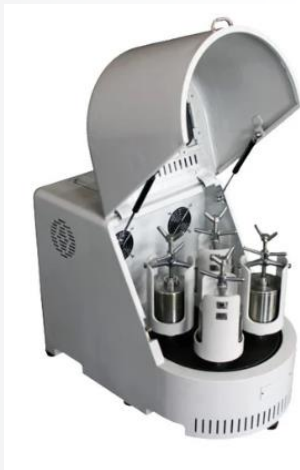
Benchtop planetary ball-mill, 20 – 40 g sample
