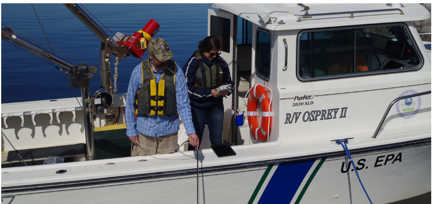
An NCCA crew measures light penetration with an underwater light meter.
