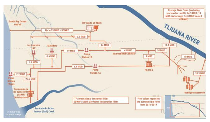
Figure 2-3 Lift stations locations near the border.
