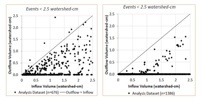
**Figure 1. Discharge volume versus inflow volume for bioretention areas with and without underdrains.** Tile A shows results for 676 monitored events across 14 individual systems with underdrains. Tile B shows results for 1,386 monitored events across six individual systems without underdrains.
