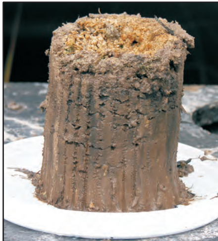
Figure 52. Everglades peat (top, organic matter 78%, WCA2A) and marl (bottom, organic matter 14%, the Park). Bottom photo also shows a benthic periphyton mat overlaying the soil core.
