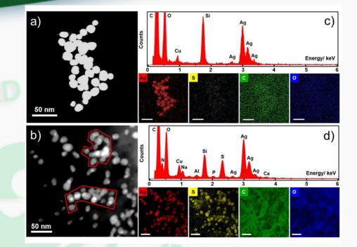
Example of STEM images and elemental mappings of pristine (a) and wastewater borne silver nanoparticles (b). The normalized EDX spectra (c, d) correspond to the highlighted areas (in red). The spectral image intensities represent the atomic fraction, and the scale bars (c, d) are identical to those in the STEM images (a, b). Source: (Steinhoff et al., 2020). Copyright: 2020 American Chemical Society.
