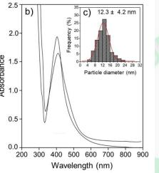
Example of acceptable TEM image, including the scale (e.g., 50 nm; a) and particle size distribution b) is from the scanning absorption spectra; c) is the mean particle diameter ± standard deviation (12.3 ± 4.2 nm) of silver nanoparticles. Source: (Sondi and Salopek-Sondi, 2004). Copyright: 2004 Elsevier.
