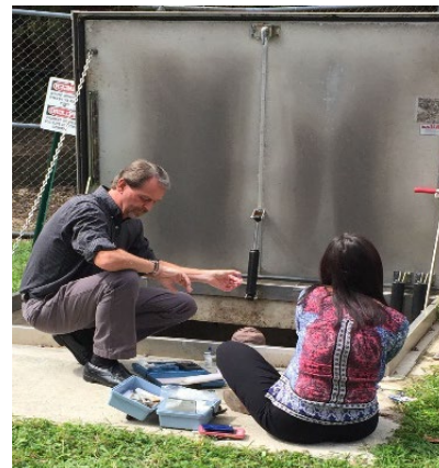
Using a field test kit to measure chlorine residual in the distribution system
