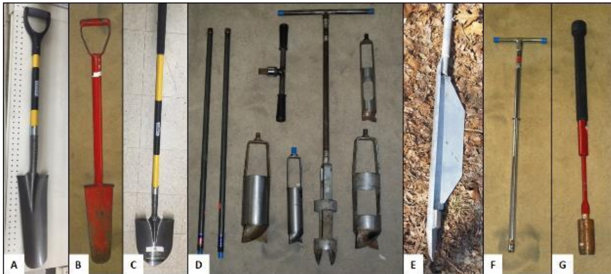
Figure 6-8. Examples of tools for Soil Pit excavation. A) Tiling spade. B) Sharpshooter. C) Shovel. D) (Left to right) Auger handle extensions, Ratchet handle, Solid auger buckets (for sand or mud), Open bucket auger with handle, and Open auger buckets (for fine textured soils). E) Peat auger head. F) Soil probe. G) Hammer corer. Photos by Frank Gibbs, Gregg Lomnicky, and Phil King.
