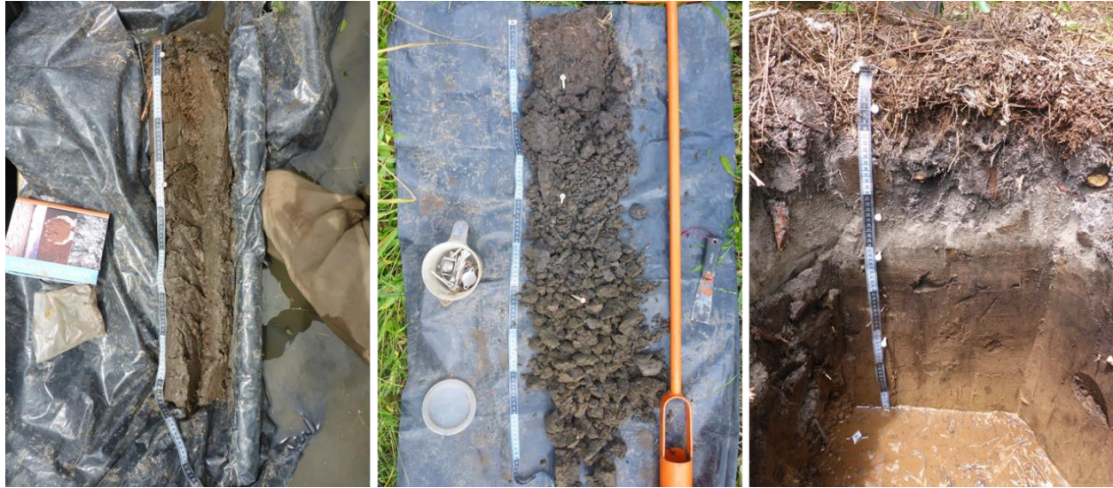
Figure D-2. Left : Soil profile described/photographed outside of the pit (extracted using a King Sampler), Middle : Soil profile described/photographed outside of the pit (extracted using augur), Right : Soil profile face photographed in the soil pit.
