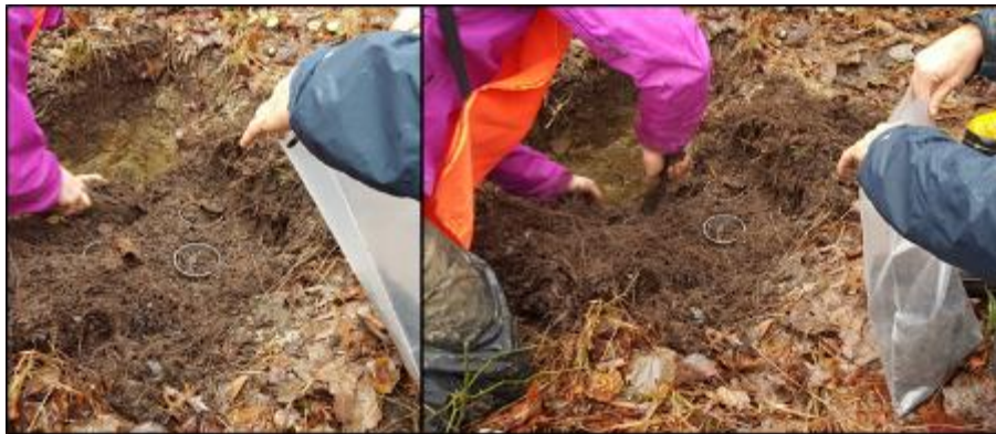
Figure 6-27. Collection of Soil Horizon Chemistry sample. Horizon Chemistry samples can be collected as Horizon Bulk Density Sample cores are extracted. Photo courtesy of Sarah Lehmann.
