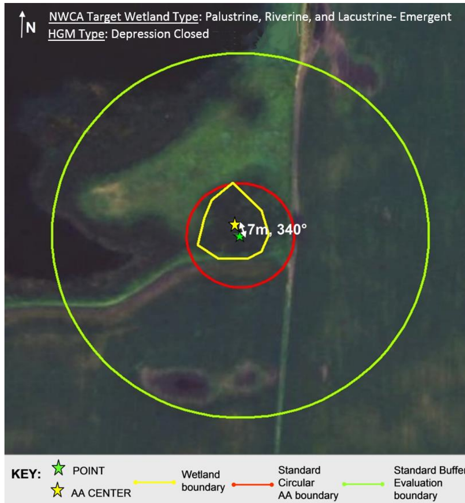
Figure 3-9. Example of a Wetland Boundary AA layout depicted on an example annotated aerial photo. Distance and bearing from the POINT to the AA CENTER are indicated. The Standard Circular AA layout and the Standard Buffer Evaluation boundary are shown for comparison.
