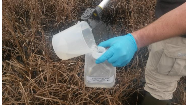
Figure 8-4. Example of filling the cubitainer. (Photo credit – Chris Turner, GLEC)
