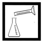
4. Use a clean graduated cylinder to take a water sample. Pour sample into a clean 125- or 250-mL Erlenmeyer flask. Dilute to about the 100-mL mark with deionized water.
