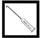
2. Insert a clean delivery tube into the titration cartridge. Attach the cartridge to the titrator body. See *General Description*, *Step-by-Step*, for assembly instructions, if necessary.
