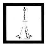
8. Add one dropper of starch indicator solution and swirl to mix. A dark blue color will develop.
