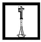
Continue the titration until the solution changes from dark blue to colorless. Record the number of digits required.
