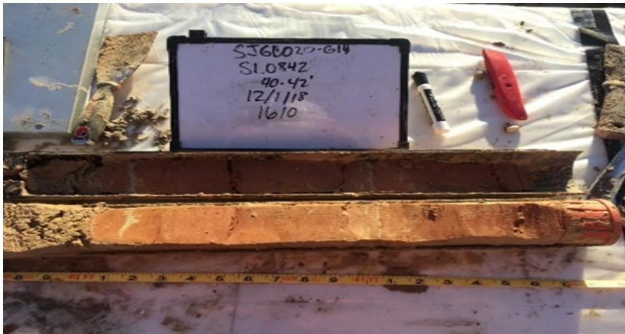
Photo 3      Figure D.3: Sample G14 (40 to 42 ft deep) in borehole SJSB-020.
