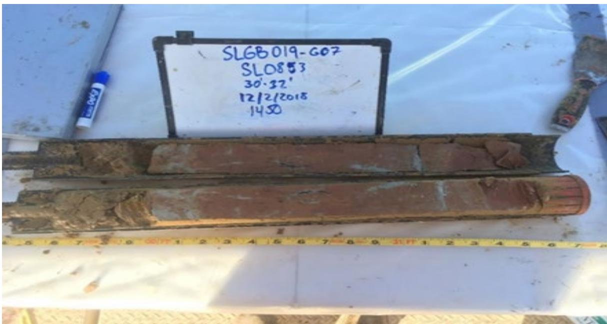
Photo 2      Figure D.2: Sample G07 (30 to 32 ft deep in borehole SJSB-019).
