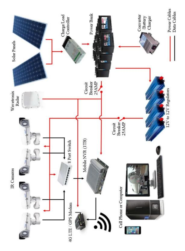
Figure 20: Schematic diagram for the Automatic Placard Recognition System
