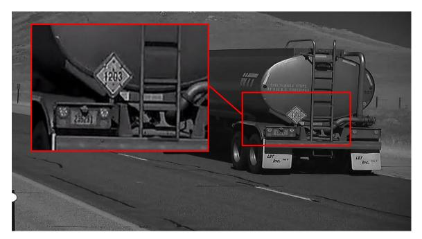
a) Image from the LPR camera pointed at the placards mounted at the back
