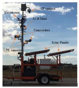
Figure 21: HAZMAT data collection trailer
