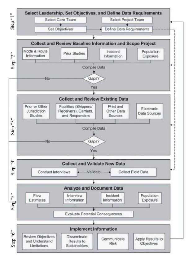
Figure 1: The HAZMAT Commodity Flow Study (HMCFS) Process<sup>2</sup>
