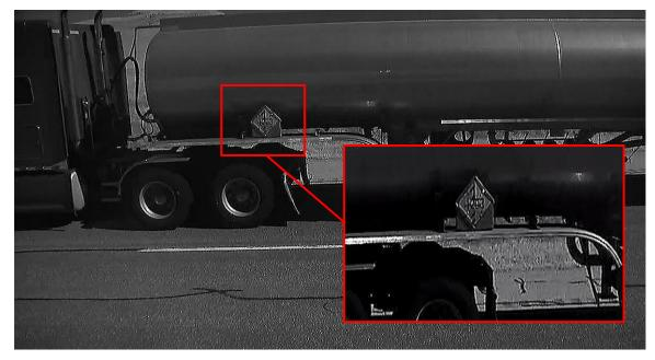
b) Image from the LPR camera pointed at the placards on the side Figure 22: Images obtained from the LPR camera
