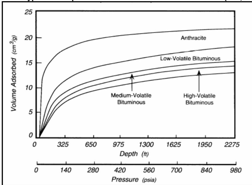
The curves shown in **Figure 4** are called adsorption isotherms because they are measured at a constant temperature.<sup>11</sup> Adsorption isotherms can be characterized by mathematical functions based on theoretical adsorption properties. One function commonly used for methane
