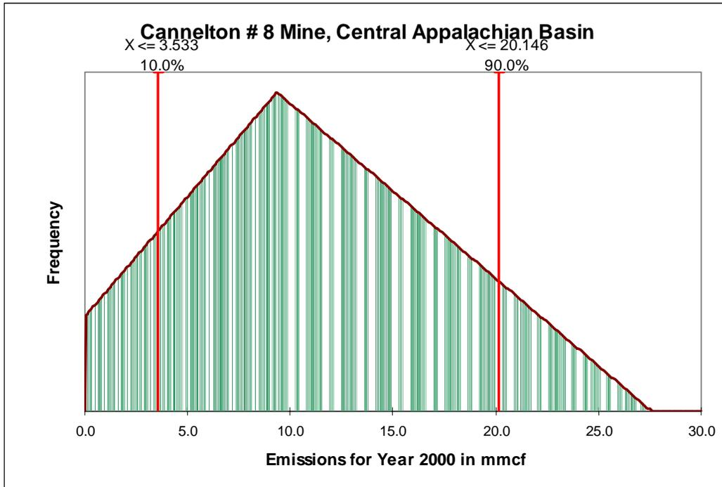
Figure F-2. Probability density function for vented abandoned mines emissions for the year 2000
