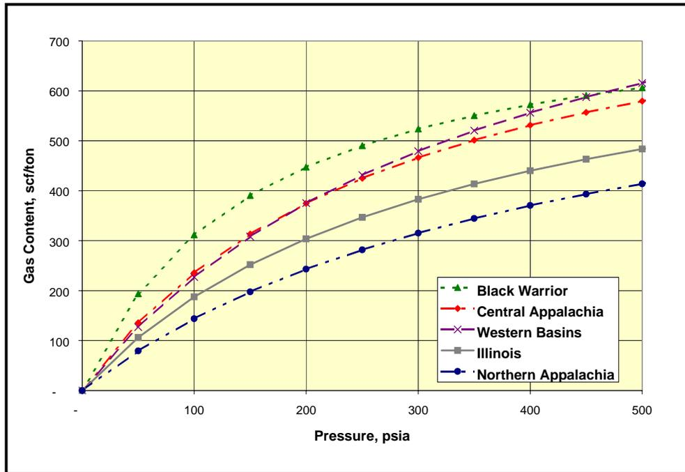
**Figure 9. Methane adsorption as a function of mine pressure for the Central Appalachian Basin**
