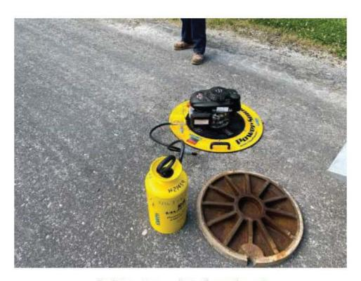
Sanitary sewer smoke testing equipment
