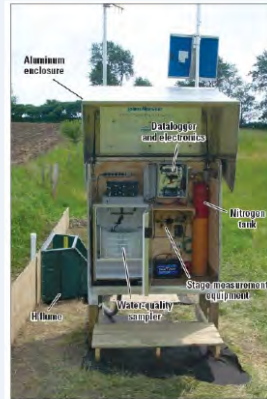
Edge-of-field monitoring stations. Left and top right, Wisconsin Discovery and Pioneer Farms (Stuntebeck et al. 2008); bottom right, Vermont (Meals et al. 2011).
