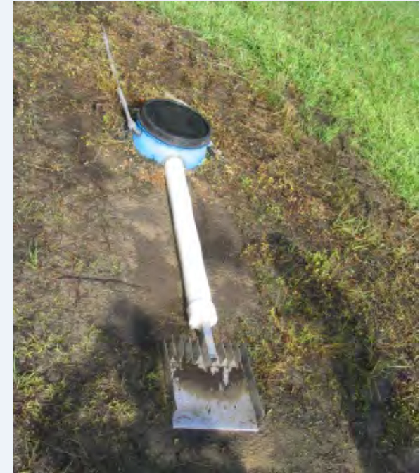
Passive runoff sampler/flow splitter, University of Georgia, Tifton, GA (photo by D. Meals, USEPA)
