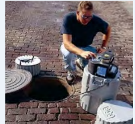
A portable autosampler (photo by Teledyne Isco, 2013)
