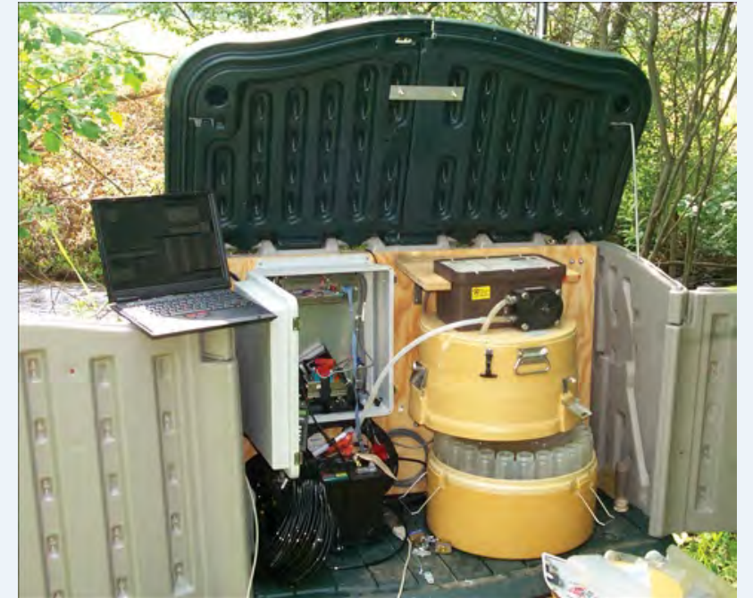
Automated sampling equipment (photo from Hall 2004)
