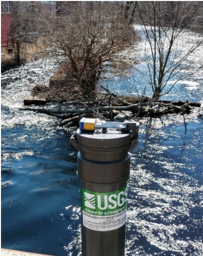
Continuous water quality monitor deployed off a bridge in Westerly, RI (photo by J. Morrison, USGS)
