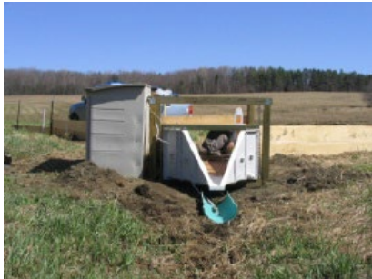
Edge-of-field monitoring station, Vermont (Meals et al. 2011)
