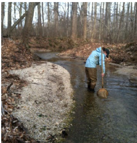
Using a D-frame net to sample a gravel-bottom stream for benthic macroinvertebrates (USEPA 2016)
