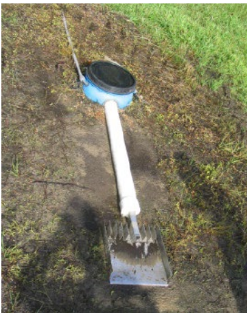
Passive runoff sampler/flow splitter, University of Georgia, Tifton, GA (photo by D. Meals, USEPA)
