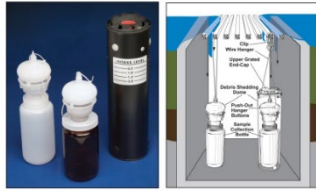
A. Nalgene® first-flush sampler. Installed below grate (at right).
