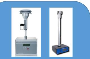
The Federal Equivalent Methods (FEMs) provide automated data at higher time resolution (generally every hour). They are used across the official air monitoring network and were designated by comparison to FRMs under typical conditions (not smoke).
