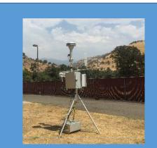
Temporary monitors also provide hourly data, were tested for performance under high concentrations, and are used extensively by government organizations for supplemental monitoring during wildland fire smoke events.
